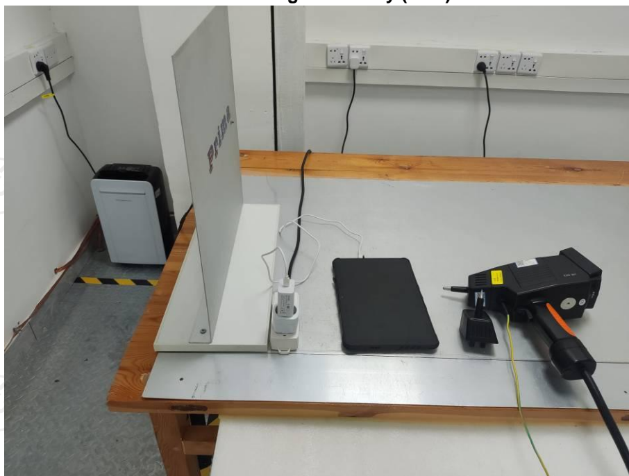
Electrostatic discharge immunity (ESD) test view
