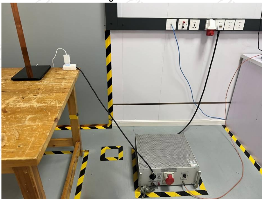
Disturbance voltage at mains terminals test view
