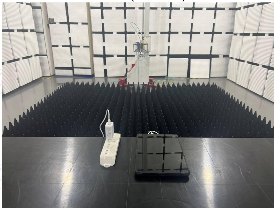
Radiated emission (1 GHz-6 GHz) test view
